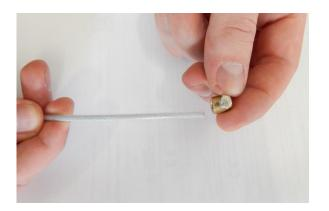
Put sleeves on the cable guides Img. 1. Place a screw in the sleeve, and best with fingers secure it until first resistance, then use flat wrench Img. 2 and make 2 full turns. Making more turns wil damage the screw head.
